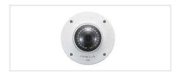
The SNC-DH260 is an outdoor vandal-resistant high definition (1080p, supporting H.264 at 30fps) 3 Megapixel mini-dome camera with Optical Day/Night function, IR Illumination, DEPA and ONVIF compliance. It supports dual streaming and triple codec encoding.
