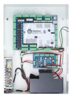
The GV-AS8111 Kit is a cabinet that contains a GV-AS8111 control panel, a power adapter board, a power supply and a backup battery case. The power supply powers the GV-AS8111 Kit as well as up to 8 output devices (12V, 0.5A per device).
