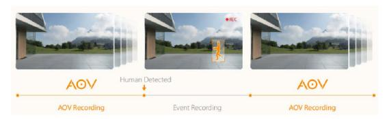
AOV PT takes it to the next level with the latest Always-on Video (AOV) technology. With AOV, the camera intelligently allocates its resources by compiling time-lapse videos from images captured at your scheduled intervals. Additionally, it also records full videos when an alarm is triggered, precisely controlling the power consumption for each operation. This enhances home safety while reducing battery consumption.
